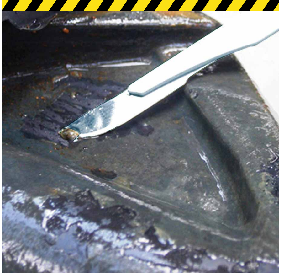
Competitor EPDM wedge after six months of operation - an example of microbiological growth on an improperly formulated rubber compound.
