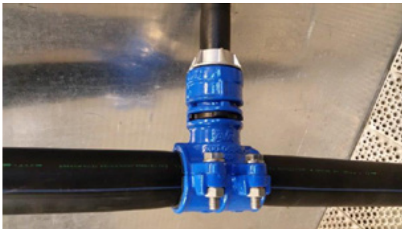
Supa Lock™ after lifetime testing is conducted.
