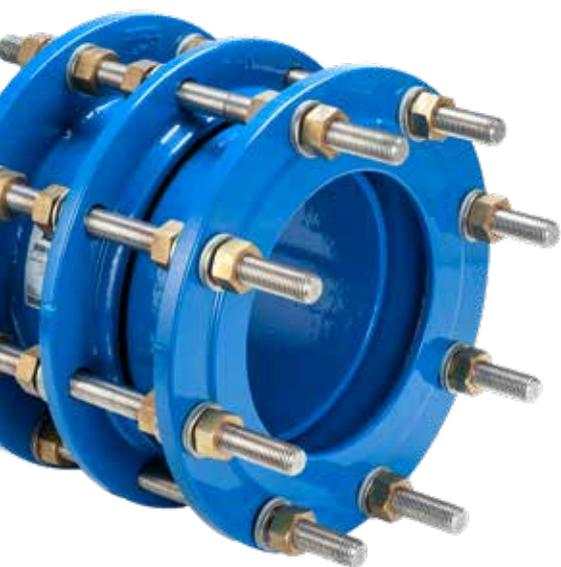
AVK dismantling joints provide easy installation and disassembly of flanged pipework and equipment and compensate for axial displacement of the pipe during installation and dismantling. The range is available in DN40-2600 in PN10/16 and up to DN1200 in PN25.
