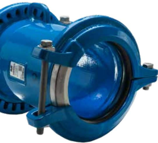
Supa One™ universal straight couplings and flange adaptors are very easy to install with only one bolt to be tightened in each end of the coupling and with the possibility of using a standard power tool. They are designed in ductile iron according to EN 545 to ensure sturdiness and durability.
